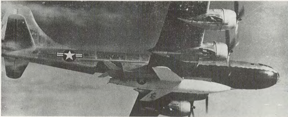
The First Rocket Ship Goes Aloft: The Douglas D-558 II "Skyrocket," the highest and fastest flying plane, nestled in the belly of the B-29 mother ship shortly before drop and ignition of the RMI 6000-series rocket engine with which it is powered.
