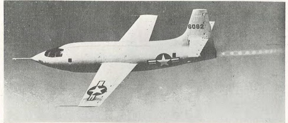
The Result: The USAF Bell X-1, first airplane to fly faster than the speed of sound; powered by the famous RMI 6000C4 rocket engine, the direct descendant of the "Sunday experiments". — (Photo courtesy Reaction Motors, Inc.)
