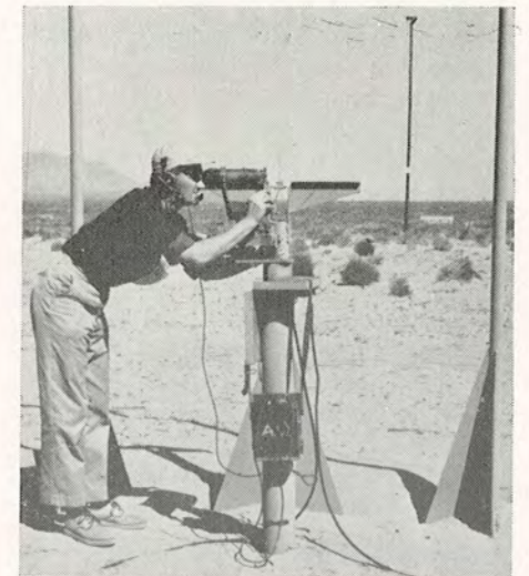
Left: The sky screen with its telescope and safety wires (too small to be seen here) manned by Robert Daly. The safe limits of flight are determined by the wires; if a rocket crosses a wire, it may land outside the range boundaries. — (U. S. Army photo.)
